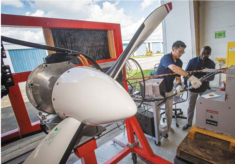
Tony Zhao and Milton Marwa connect the battery cable to an experimental engine and prop at the Eagle Flight Research Center in Florida. Above right: Victoria Li and Marwa work on an airframe for the hybrid engine project.
